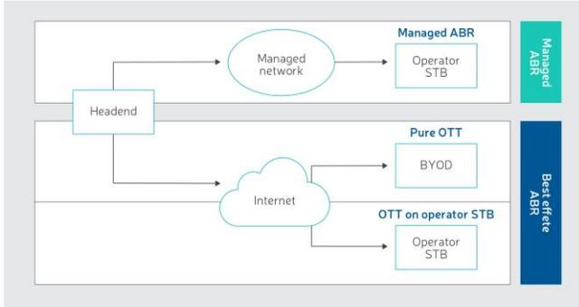
FIGURE 1: UNICAST NETWORK TYPES.
