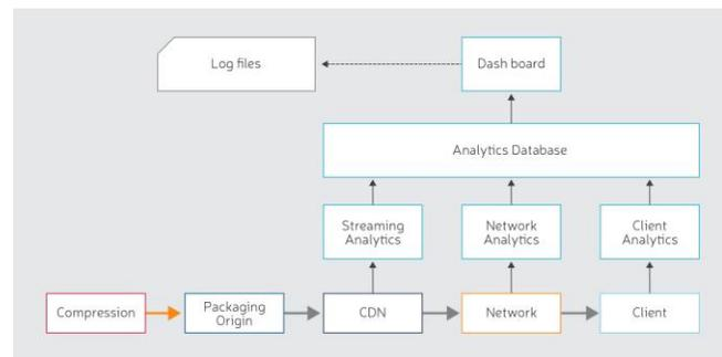
FIGURE 6: GENERIC NETWORK MONITORING SOLUTION.
